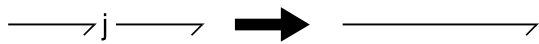
FIGURE B.2 Elimination of junctions ( j can be a 0-junction, a 1-junction or a M-junction )
